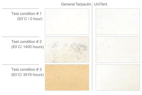
As proven by the weathering test, UniTent is durable and long lasting PVC coated fabric and it is your perfect choice for outdoor tent and architecture usage .
