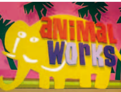
GATORFOAM® laminated and cut to shape with a jigsaw
