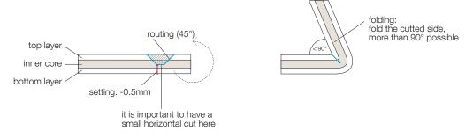
The specific settings need to be tested for each machine and thickness.
