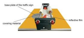
If it is necessary to apply two pieces of prismatic sheeting side by side (splicing), they must not overlap. Depending on the format, the gap should be approximately 1 mm [0.04 inches]. Please make sure that a right side of the film web is always bonded to a left side, thus ensuring the uniform orientation of the film's honeycomb structure (shown below).
