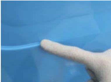
Apply the film with a wet glove only on the edges (first on the upper side and then on the lower side of the corrugation).
