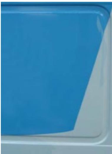
**The finishing effect is to reheat the wrapping in the final step to reduce the memory effect on the vinyl.**
