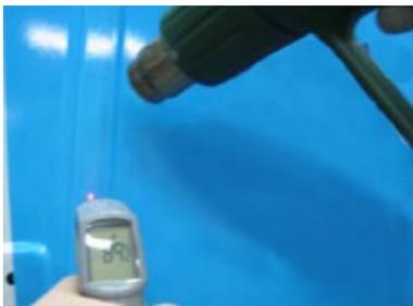
Reheat the corrugated surface. Increase heat temperature of up to 85 - 105°C. If the temperature for the final tempering process is lower the memory effect stays within the film. These high temperatures are needed to create a new form for this vinyl. It is absolutely recommended to use a infrared thermometer to avoid any failures in measuring the surface temperature.
