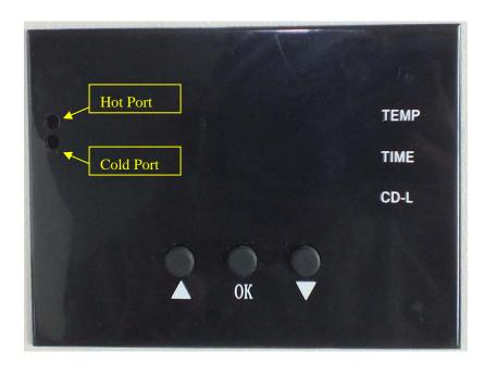
There are two buttons under the cover, one is "hot port", and the other is "Cold port". If the real temperature is lower than digital controller shown, you can adjust the "hot port"; Clockwise to Raise temperature; anticlockwise to low temperature.
