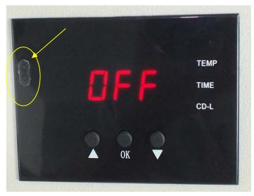
Use the screwdriver to open the plastic cover which marked in Red.
