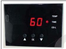
Press button after temperature setting and the time light is on. Select with arrows the time according to different transfer
