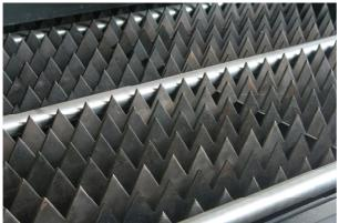
The movement system adopt the drive system of high precision ballscrews and servo motor, and this assure the high precision of the cutting. Serrate platform and trim strip are very suitable for cutting metal sheets. The user can put in and take out the materials faster and easily.
