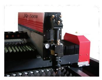
Our solid laser cutting machine uses USA imported mechanical following cutting head. Cutting head laser nozzle locking ring touch the metal sheet materials surface, cutting head move up and down, and it can achieve same focal cutting. The cutting head has high sensitivity, stable running and good reliability. When cutting metal sheet, there is no obvious sparks flying phenomenon, and avoids the lower sensitivity and failure caused by air dielectric changing and
