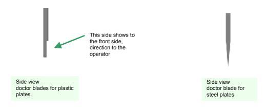
Important: The blade edges are very sharp. You will get injured, especially when touching the edges of either of the blade types for steel plates.
